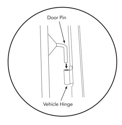
Hold the door straight out from the vehicle with the hinge pins over the body hinges.
