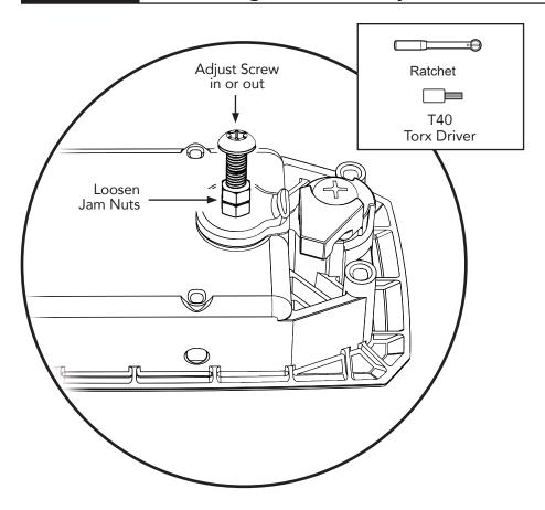
The Paddle Latch mechanism can be adjusted using the Screw and Jam Nuts that you installed in Section 1, Page 4.
