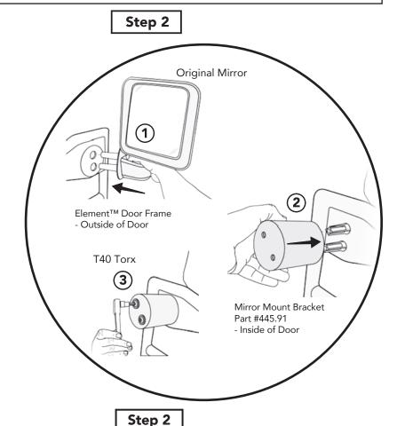
The mirrors from the original doors can be mounted to the Element<sup>™</sup> Door using the Mirror Mount Brackets #445.91.
