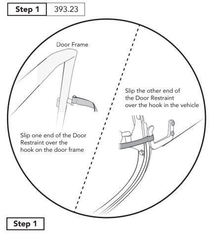
Locate the two (2) Door Restraints # 393.23. Slip the loop in one end of a Door Restraint over the hook on the door frame.
