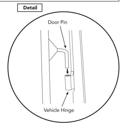
Hold the door straight out from the vehicle with the hinge pins over the body hinges.
