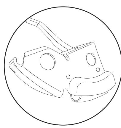
Insert a Grommet into the bracket at the end of the #6 Bow Assembly.
