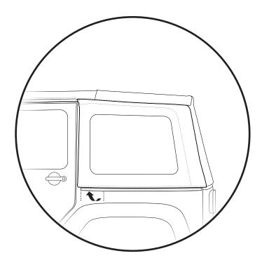
Tuck just the first couple of inches of the plastic strip along the bottom edge of the Quarter Window under the Jeep belt rail.
