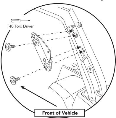
Attach the #6 Bow Support brackets to the sport bar down tubes. Place one pin in the small hole above the lower threaded insert in the sport bar and place the other pin in thescrews slot above the upperv threaded insert. secure with two (2) M8  $\times$  28 mm screws.
