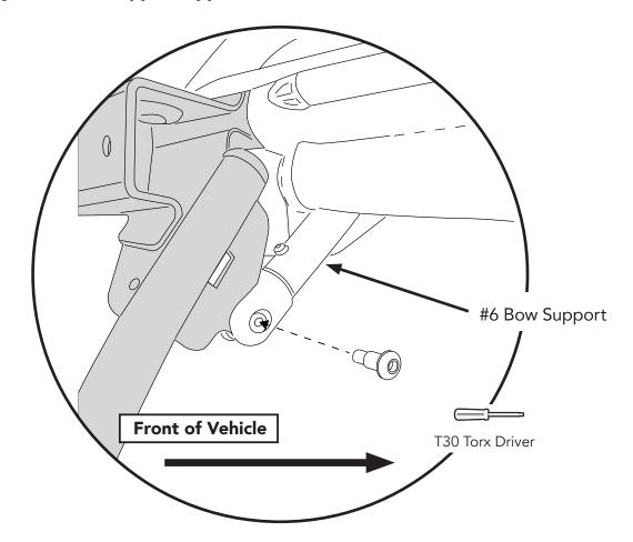
Pull the #6 bow down over the rear of the vehicle then attach the #6 Bow to the #6 Bow Support using one (1) Pivot Knuckle Screw per side.
