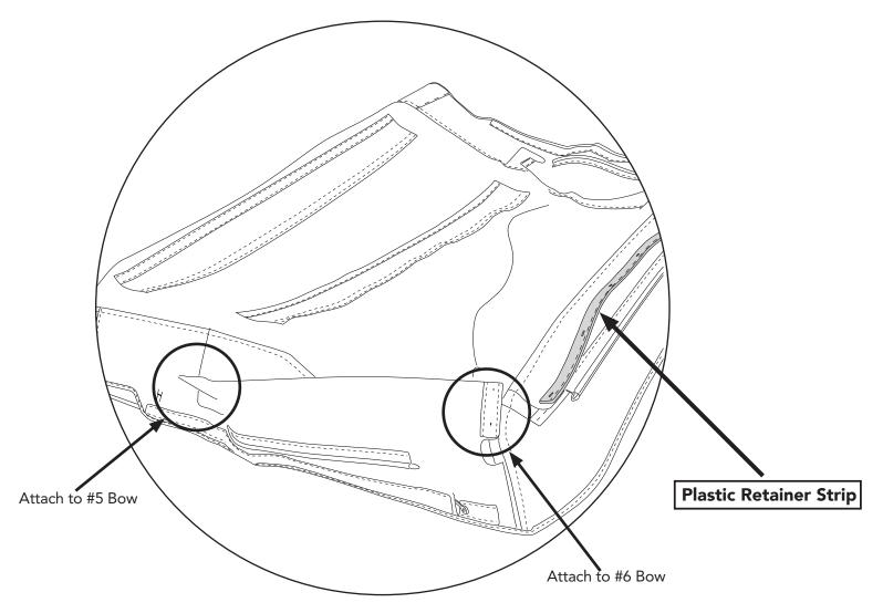
Lay out the Top Fabric Assembly with the inside facing up.
