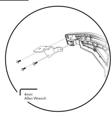
Attach the #4 Bow Bracket Left to the Left Side Door Rail Assembly using three (3)  $M6 \times 1 \times 14$  Button Head Socket Cap Screws.
