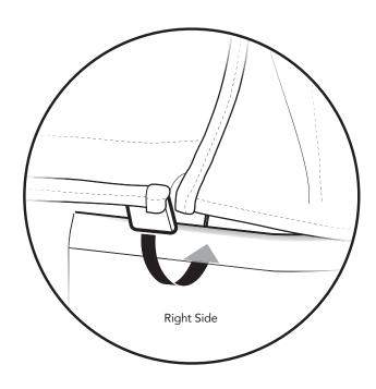
Tuck the plastic tabs at the bottom corners of the Rear Window under the Jeep belt rail.
