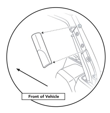
Snap off the trim panels on the rear down tubes of the sport bar.
