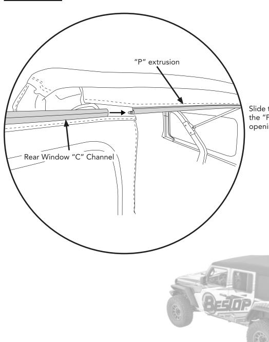
Slide the "C" channel from the top of the Rear Window onto the "P" extrusion located along the top of the rear window opening on the Top Fabric assembly.
