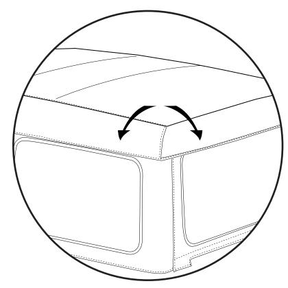
Fold the rear corners of the top down and connect the hook and loop across the top of the side panels.
