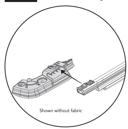
Align both ends of the Tailgate Bar in the openings of the Tailgate Bar Retainers on the vehicle.
