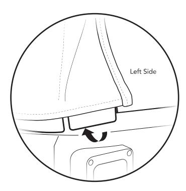
Tuck the plastic tab at the bottom rear corner of each Quarter Window under the Jeep belt rail. Roll the tab on each side up underneath the Jeep belt rail.
