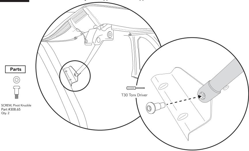
Attach the #6 Bow Support to the #6 Bow Mounting Brackets using one (1) Pivot Knuckle Screw per side.
