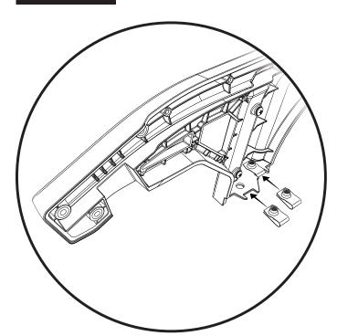
Attach the two (2) U-Clips to the Upper Rear Door Rails in the positions indicated. Make sure to have the threaded barrel of each U-Clip facing up.
