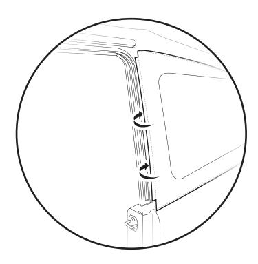
Locate the the sewn-in plastic strip along the front edge of the left Quarter Window.
