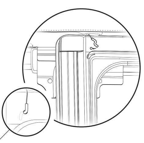
Locate the Z-Clips, which extend out from the edge of the top fabric just above the Door Rail on each side of the Jeep.
