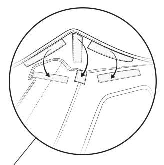
Locate the Hook & Loop strips at the rear corners of the top fabric.
