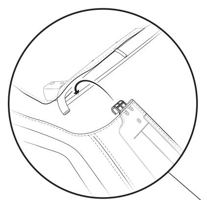
Attach the Quarter Window Stiffeners (attached to the inside of each Quarter Window) to the #4 Bow cross bar.
