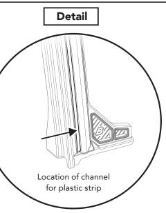
Locate the the sewn-in plastic strip along the front edge of the left Quarter Window.
