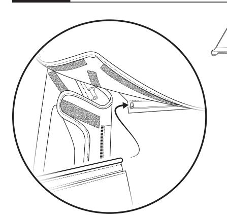
Lift up the corners of the Top Fabric to expose the Rear Window attachment channel.
