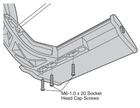
Adjust the Step from side to side. Make sure to leave clearance for foot access to lower step. Tighten the allen head bolts.
