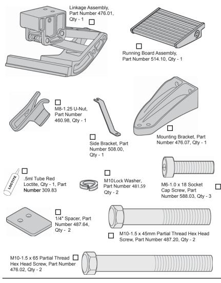
Apply 2 drops of loctite to each fastener before installtion.
