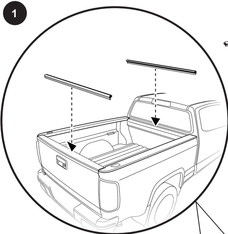
Place the Front Rail and Rear Rail onto the truck bed.
