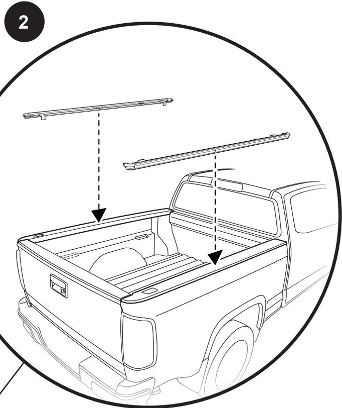
Place Side Rail assemblies onto the the truck bed. Lay the Rails on top of the plastic bed protectors.
