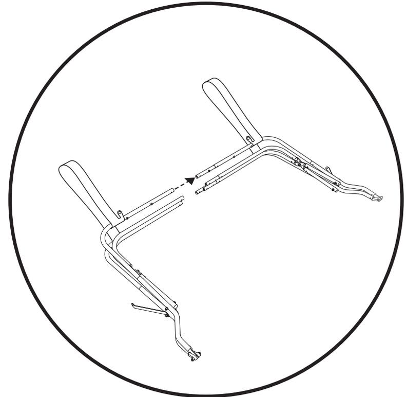
Attach Driver Side Bow Stack to the Passenger Side Bow Stack.
