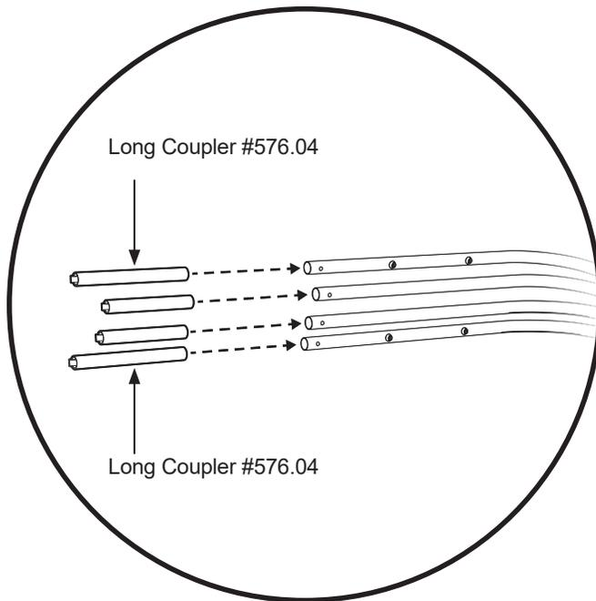
Attach Bow Couplers to the Passenger Side Bow Stack.
