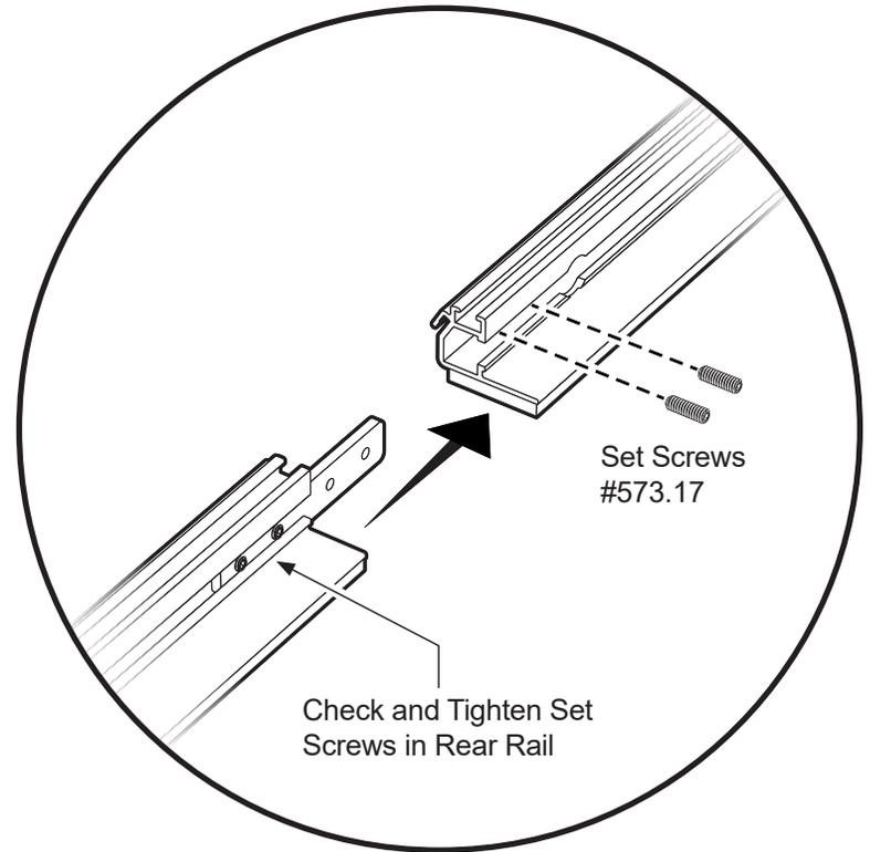
Check and Tighten Set Screws in Rear Rail
