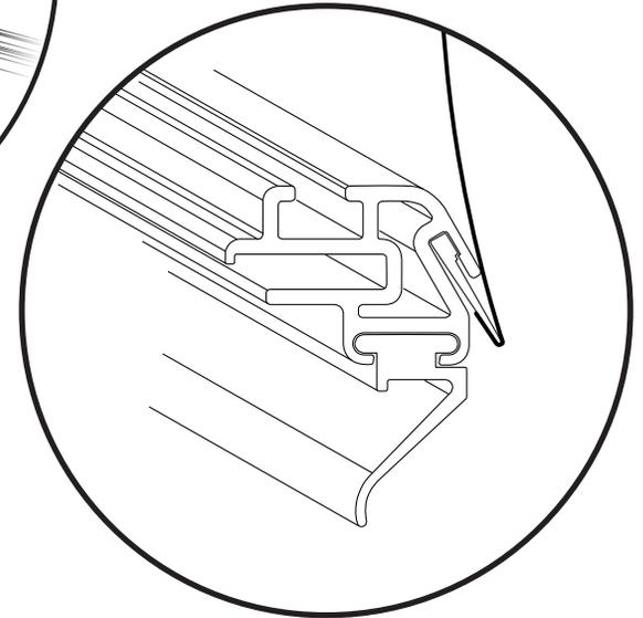
Slide the front rail onto the plastic retainer at the bottom of the front window. The rail should go under the large flap.
