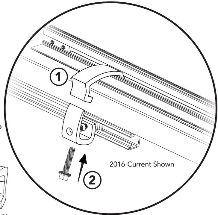
① Remove the end cap from the vehicle track system, and slide the Track Block into the track.
