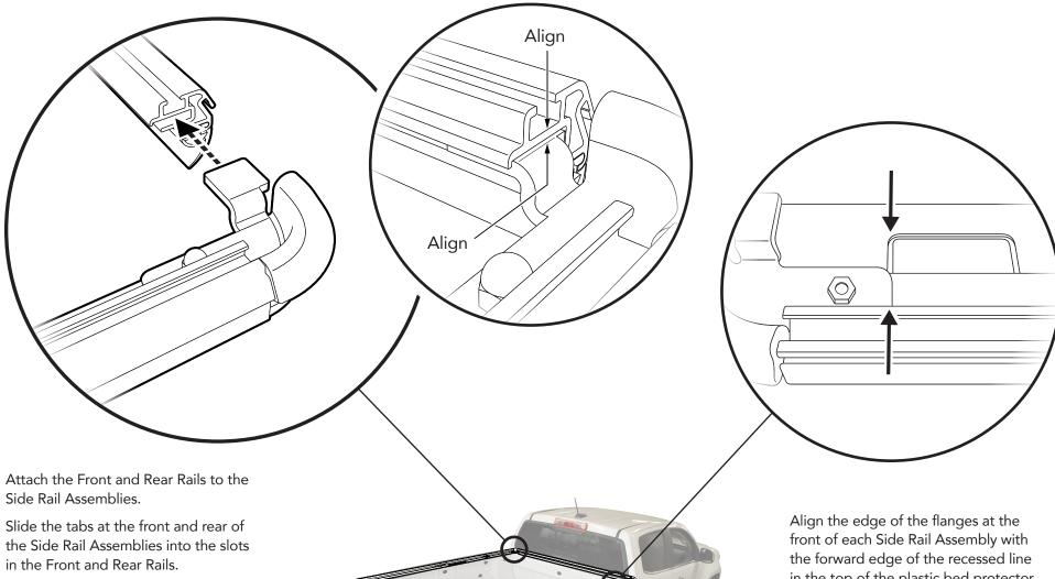
Make sure that the ends of the Front Rail and Rear Rail extrusions are aligned with the tongue of the attachment feature, where the tongue bends, and the small corner protrudes.
