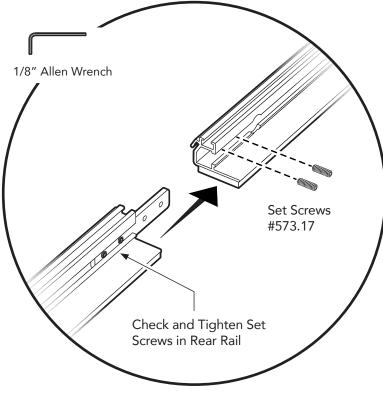
Assemble the Left Front Side Rail and the Left Rear Side Rail.
