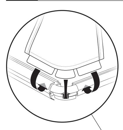
Tuck the plastic tabs at the bottom of each corner of the top into the slots in the Side Rails and Front and Rear Rails.
