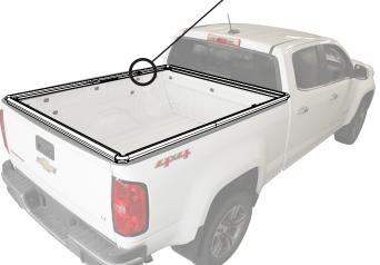
1 Attach Clamp Pads to the Upper Clamps on the Front Side Rails, on the rib farthest from the rail.
