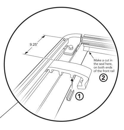
Adjust the Side and Front and Rear Rail assembly right-to-left to center it on the bed width.
