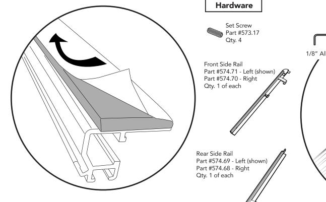
Locate the Foam Tape on the Left and Right Side Rails, and remove the paper backing from the foam tape.
