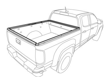
Attach Driver Side Bow Stack to Passenger Side Bow Stack.
