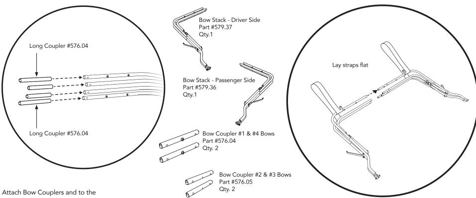
Attach Bow Couplers and to the Passenger Side Bow Stack.
