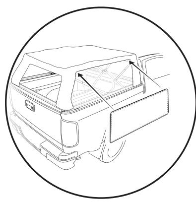
For easier access to the zippers, you may want to lift the corners of the top onto the roof fabric.
