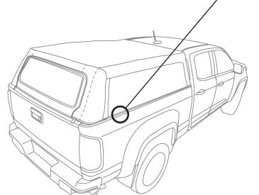
Tuck the plastic tab along the bottom edge of each Side Curtain into the slot along the side of each Side Rail.
