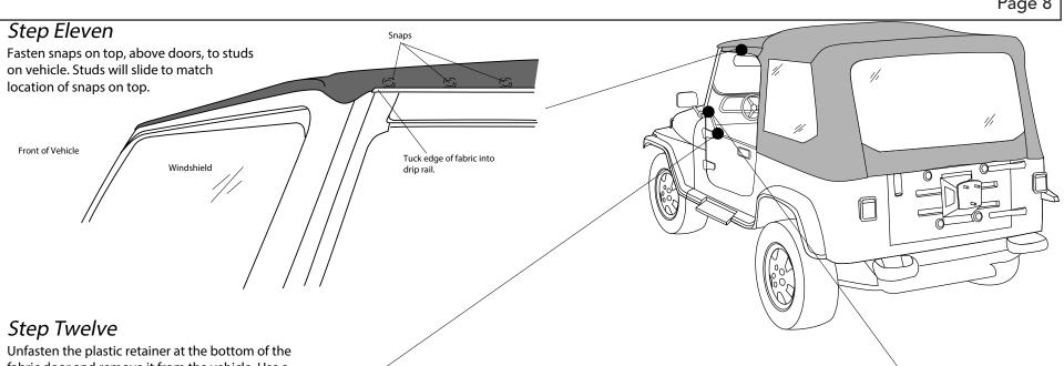
fabric door and remove it from the vehicle. Use a razor knife to cut the stitches on the old door covers and remove them from the door frames.
