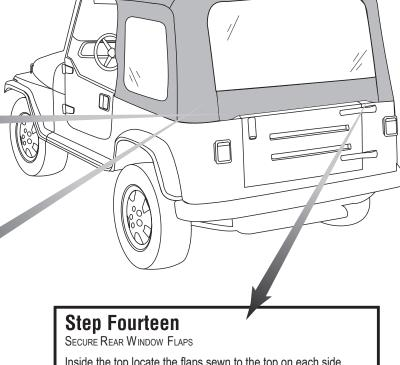
Inside the top locate the flaps sewn to the top on each side of the rear window opening. Pull the flaps over to cover the zipper and tuck them in.
