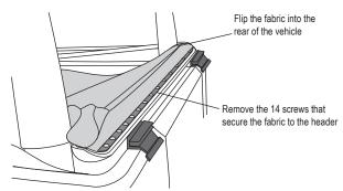
Manufacturing Note: Due to a recent header assembly modification by Daimler Chrysler, the plastic strip on the windshield header may have 8 screw locations instead of 14. Both attachment numbers of screws will securely fasten the header and perform as the original design was intended.
