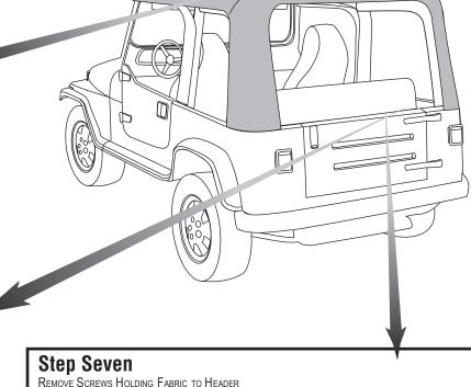
Flip the top fabric back over into the rear of the vehicle (so that the fabric lays backing side up) to expose the plastic strip along the edge of the fabric. Remove the fourteen screws that secure the fabric to the header, setting the screws aside for use in installing the new top. Then remove the old top fabric from the vehicle.
