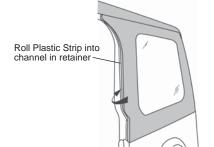
Locate the two plastic strips sewn to the sides of the top, above each door. Slip the strips into the channel in the Door Surround above the door opening. It is easiest to insert the front plastic strip into the channel first.
