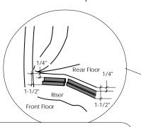
**Note:** After drilling the holes for the "Z" Channel in the floor riser, put silicone sealer on the holes before installing the channel with the screws.
