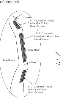
Warning: Check for wiring and fuel lines before drilling holes in riser.
