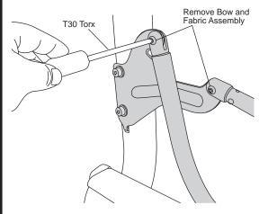
Release the front of the top from the windshield and lay the bows down. Refer to owner's manual for instructions.
