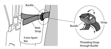
Note: Do not wrap the straps around the seat belt
