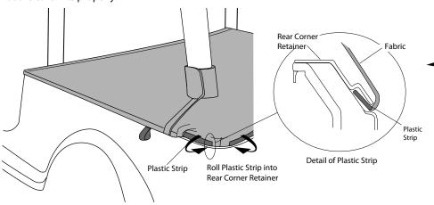
Note: The Plastic Protector sewn into the fabric must be located to minimize abrasion between the Duster Cover and the Tailgate Retainer Mounts.
