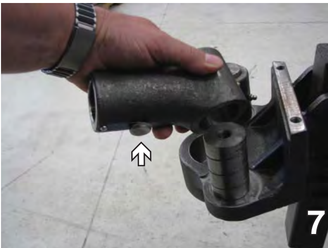
7. Grease the new trunnions, with the pin down slide on.
