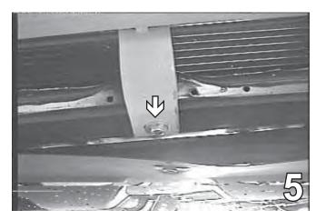
5. Use the 3/8" -16 x 1 1/4" hex bolts and 3/8" whiz nut with 14" wire for the lower brace, tighten the nut and the bolt. Use LOCTITE red with each bolt throughout the installation.
