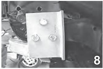
8. Once the middle braces are bolted to the frame, drill the 3/8" holes for each side. Use the 3/8"-16 x 1 1/4" hex bolt, 3/8" lock washer, and 3/8 flat washer.
