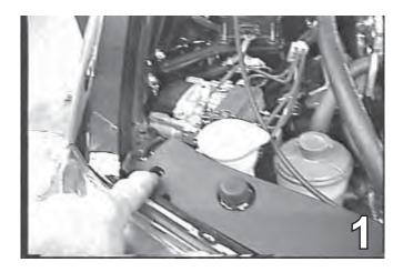
Open hood and remove pushpins from the top of the grille and set aside to be reinstalled later.
