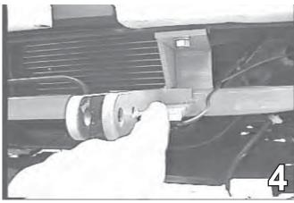
4. Hold the baseplate up so it straddles the frame and the front braces lay flush to the bottom of the metal bumper and the center brace lines up to an existing hole in the lower cross member.
