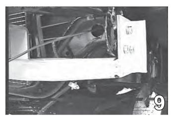
Insert the wire nut plate through the large hole on the cross frame. Tighten bolts according to the chart on the front page of this document.  Replace the electrical connections, bumper and fascia. Baseplate installation is now complete.
