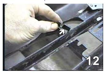
12. Trim off the plastic tabs on the back side of fascia. These are found near the grille opening area that attachment tabs will go through. Do this to both sides of the vehicle.
