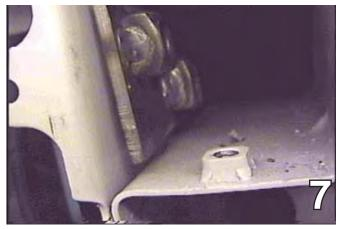
7. Hold baseplate to align with 17/32" drilled holes and insert the 1/2" nut plate, passenger's side into the frame end. Hand tighten the 1/2-13 x 1 1/2" hex bolts and the 1/2" lock washers. Do this to both sides of the vehicle. Reinstall metal bumper with existing metric bolts and clamp baseplate to the bottom of the metal bumper with the vise grips. Tighten 1/2-13 hex bolts with the 3/4" socket. Do this to both sides of the vehicle. **Be sure to apply LOCTITE Red to ALL bolts.**
