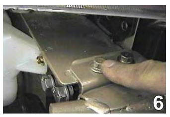
Unclamp baseplate and set a side. Using the 12MM socket, remove the two metric bolts on top and one on the bottom of the metal bumper. Do this to both sides of the vehicle. Pull forward and set metal bumper and bolts aside to be reinstalled later.
