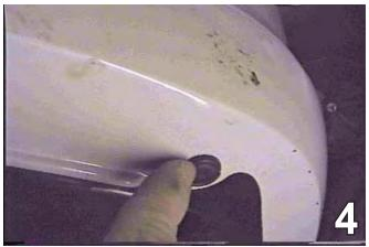
4. Remove four pushpins on the bottom side of the fascia. Pull fascia corners out to the side of the vehicle then forward to release. Set fascia and bolts aside to be reinstalled later.
