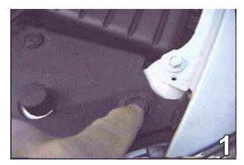
1. Remove ten pushpins from the top edge of the front fascia. Set pushpins aside to be reinstalled later.
