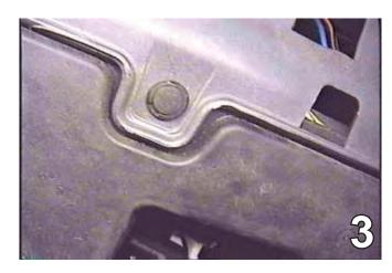
3. Remove four push pins from the bottom side of the fascia.
