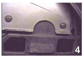
Using the Phillips screw driver, remove four screws from the bottom side of the fascia, just forward of front tire. Pull the fascia forward. Set it and the screws aside to be reinstalled later.
