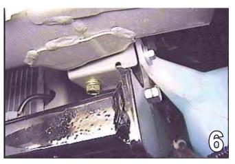
Remove the three metric bolts from the wind shield washer reservoir with the 10MM socket, unplug. Set aside to be reinstalled later.
