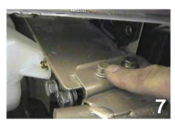
7. Hold the baseplate up to the bottom of the metal bumper, align with forward reservoir bolt and clamp with vise grips. Using the 3/8" transfer punch, mark all drilled holes. Remove the six metric bolts from the metal bumper with the 12MM socket. Set aside to be reinstalled later.
