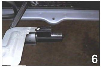
6. Using the small flat screwdriver, remove the temperature sensor and set out of the way to be reattached later.
