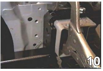
10. Set the baseplate in place on the frame ends as shown. Slide it as far back as possible and clamp it with the large vise grips. Do this to both sides of the vehicle.
