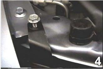
Using the 10MM socket, remove two metric bolts just above the headlight assembly. Do this to both sides of the vehicle. Set the bolts aside to be reinstalled later.
