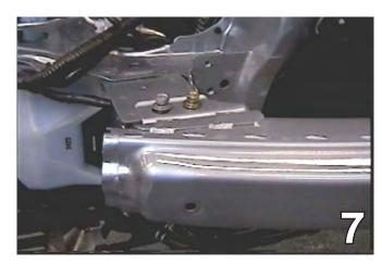
7. Using the 12MM socket, remove two metric bolts from the top of the metal bumper and one metric from the bottom. Set the bolts and the metal bumper aside to be reinstalled later.
