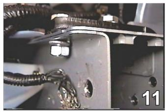
11. Using the baseplate as a template, drill the top two holes with the 13/32" drill bit. Do this to both sides of the vehicle. Install the 3/8-16 x 1 1/4" hex bolt, 3/8" lock washer, and the #10-32 hex nut into the frame end to align with the drilled holes and tighten the 3/8-16 x 1 1/2" hex bolt and lock washer. Be sure to apply LOCTITE Red to ALL bolts before tightening. Tighten ALL bolts according to the torque chart in the Baseplate General Towing Instructions.
