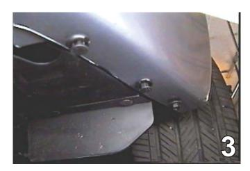
Remove the four metric bolts from the bottom edge of the front fascia with the 10MM socket and seven pushpins. Pull the fascia forward, set it and the pushpins aside to be reinstalled later.
