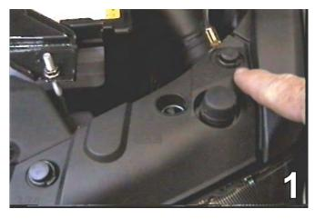
Remove the twelve pushpins from the black plastic cover on the top side of the fascia. Lift the cover and set it and the pushpins aside to be reinstalled later.
