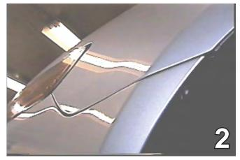
Remove one Phillips screw from the fascia's corner, just above the front tire. Do this to both sides of the vehicle.
