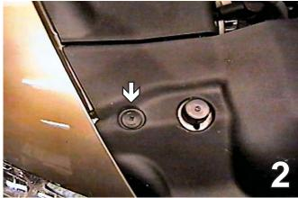
Remove one pushpin outside of the hood bumper. Do this to both sides of the vehicle. Lift up the black plastic cover from top side of the fascia and set aside.
