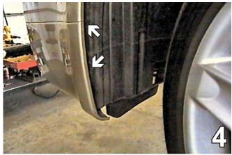
4. Just forward of the front tire are two pushpins to remove. Do this to both sides of the vehicle.
