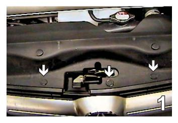
Just forward of the hood latch are three pushpins to remove from the top of the fascia. Set push pins aside to be reinstalled later.
