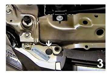
Remove the pushpin from the top edge of the fascia just inside of the headlight assembly. Do this to both sides of the vehicle.
