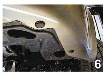
Just forward of front tire is one metric bolt to remove with the 10MM socket and one push pin. Do this to both sides of the vehicle.
