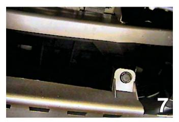
7. Remove two push pins from the lower edge of the front fascia, just below the license plate. Set bolts aside to be reinstalled later.
