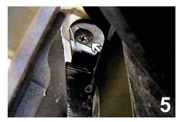
Pull wheel well cover away from the fascia edge and remove the Phillips screw from the fascia's corner with the Phillips screwdriver. Do this to both sides of the vehicle.
