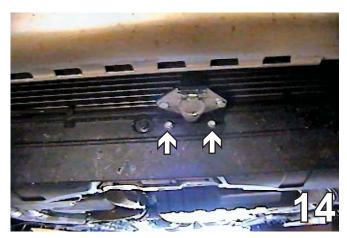
14. Using the two self tapping screws, install the electrical bracket just below the fascia on radiator cross member as shown in the photo above.
