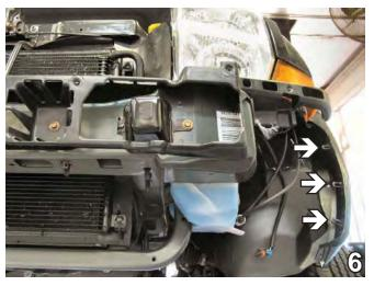
6. Release the three clips from inside of the wheel well, just forward of the front tire, on the fender guard. Disconnect fog lights (if applicable). Pull forward on the fascia and set it aside carefully to be reinstalled later.
