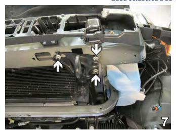
Using a 15MM socket, remove three metric nuts from the tow hook. Do this to both sides of the vehicle. The tow hooks will **NOT** be reinstalled, make sure that these are returned to the customer.
