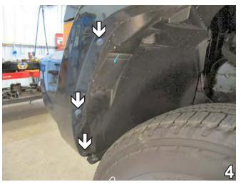
Just forward of the front tire, inside the wheel well, remove three rivets with the diagonal cutters. Discard rivets as new rivets are provided for reinstallation of the fascia.
