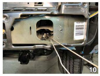
10. Install the backing plate onto the hex bolts followed by the 3/8-16 nut plates by inserting them through the frame cup opening and aligning with the bolts.
