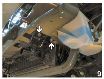
9. Align the baseplate with the two outside existing holes, where the tow hooks were connected to the frame rail, and clamp in place with the vise grips. Insert 3/8-16 x 1 1/4" hex bolts with 3/8" lock washers. Do this to both sides of the vehicle.
