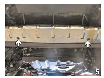
Using a 10MM socket, remove two metric bolts on the bottom side of the fascia. Set bolts aside to be reinstalled later.
