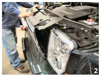
Pull up on the black plastic on the top of the fascia to release. Lift grille straight up to remove. Set grille aside to be reinstalled later.
