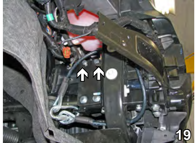
19. On the top of the support plate, insert 3/8"-16 x 1-1/4" hex bolts with 3/8" lock washers and attach to 3/8-16 lock nuts. Be sure to use Loctite Red on all the bolts. Do this to both sides of the vehicle.
