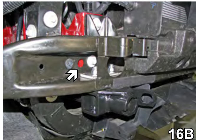
16B. MODELS WITHOUT TOW HOOKS: Insert the two (2) 3/8"-16 x 4 hex bolts with 3/8" lock washers, spacer plate (24), 3/8" flat washers and 3/8-16 hex nuts. Be sure to use Loctite Red on all the bolts. Do this to both sides of the vehicle.
