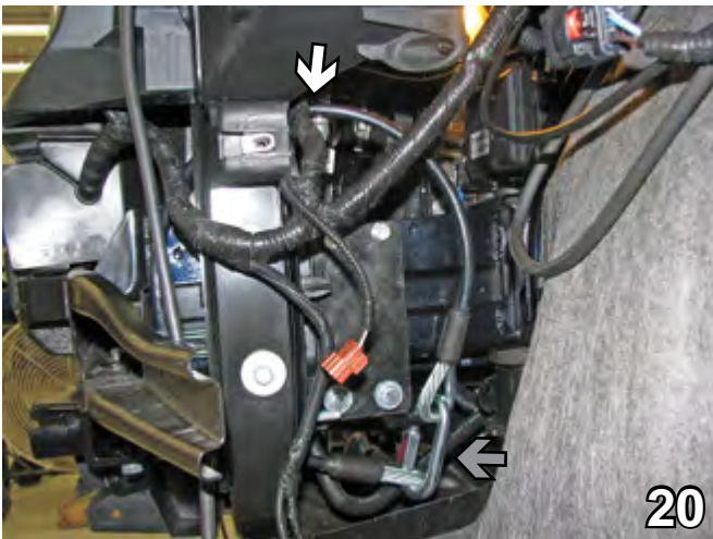
20. Attach the permanent baseplate safety cables to the provided convenience link on the baseplate (gray arrow). The photo above shows the recommended installation of the cables to frame of vehicle (white arrow). Additional options may interfere with suggested mounting; in this case secure the cables to a solid piece of the frame as described in the instructions included with the permanent baseplate safety cables. Be sure the safety cables do not rub against any hoses or moving parts. Do this to both sides of the vehicle.
