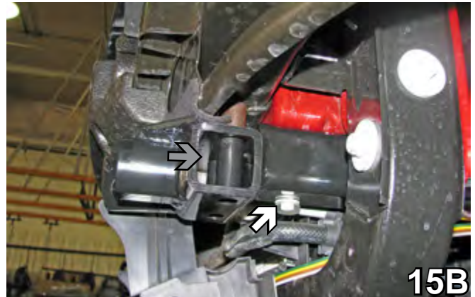
15B. MODELS WITHOUT TOW HOOKS: Insert (2) 107-3191 into place (gray arrow) before installing 10MM bolts (white arrow). Do this to both sides.
