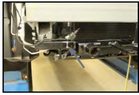
5. On the passenger's side, remove the push pins that hold the temperature sensor in place. Gently set it over to the side of the vehicle until after the baseplate has been installed. Once the baseplate has been installed, put the push pins on the side and front back to the original location. Using a cable tie, secure the temperature sensor to the baseplate.
