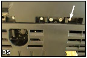
On the underside of the vehicle, towards the center, there are three (3) 10mm bolts that need to be removed. Two (2) are located towards the center and one (1) is located towards the outer edge of the Passenger's side.
