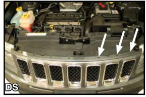
With a 20 Torx remove the seven (7) bolts that are located on the top portion of the fascia. There are four (4) on the Passenger's Side and three (3) on the Driver's Side.
