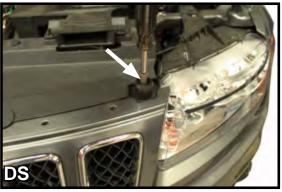
2. With a 27 Torx remove the two (2) bolts that are located on the upper side of the vehicle, one (1) per side.
