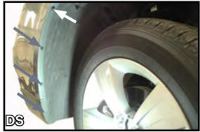
3. Using a 10mm socket (white arrow), remove the top bolt in the front wheel well area. The other three (3) bolts (grey arrows) require a 7mm socket.
