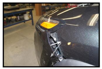
Lift the corners of the fascia up towards the fender (white) and out to release (gray).
