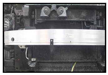
9. **Optional:** If installing a breakaway, screw the breakaway bracket to the bumper at the desired location with the #10-16 x 1" self drilling screw. Attach the breakaway to the bracket with a 1/4"-20 x 3/4" bolt and 1/4"-20 lock nut.
