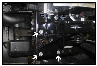
7. Install the baseplate to the vehicle using the three (3) existing extension bolts (white). Install 10MM-1.25 x 40MM bolts with 3/8" flat washers and 10MM lock washers into the lower bumper bolts (gray). Fully tighten all fasteners. Do this on both sides of the vehicle.
