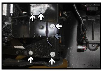
6. Using a 15MM socket, remove the three (3) bolts from the frame extension and two (2) bolts from the bottom side of the bumper (white). Using a 10MM socket, remove the nut from the fascia extension (gray). Do this on both sides of the vehicle. The extensions will not be reinstalled.
