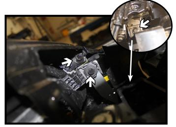
2. Using a 10MM socket, remove the three (3) screws from the backside of the fascia next to the fender. There are two (2) in the corner and one (1) directly below the bracket (inset). Do this on both sides of the vehicle.
