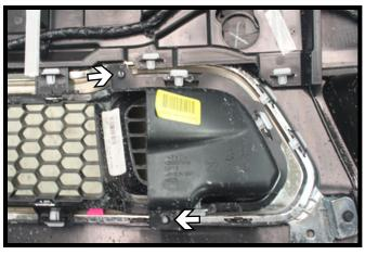
10. Using a 7MM socket, remove the two (2) screws from the cover on the backside of the fascia and unsnap the cover from the fascia. Do this on both sides of the fascia. The covers will not be reinstalled.
