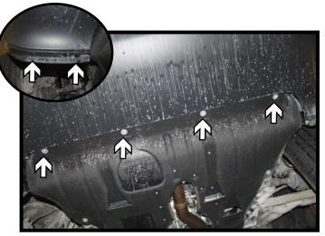
4. Remove the four (4) rivets from the underside corners of the fascia (inset). There are two (2) on each side. Using a 10MM socket, remove the four (4) screws from the middle portion of the fascia.
