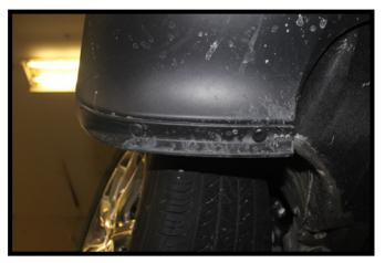
12. Install the new plastic rivets into the underside of the fascia, where the factory rivets were removed.
