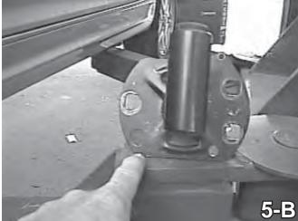
5. Remove the two front bumper brackets. There are three nuts holding each piece. The pop rivets need to be drilled out. The lower ridge where the pop rivet is will need to be trimmed off. Set the nuts aside to be reinstalled later.
