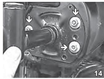
14. Drill one 3/8" hoe between the two nuts on the outside of the brackets and one below the lower nut. Also drill one hole below the nut on the inside of the bumper bracket. Use the 3/8" hardware as shown in the drawing on page 2. Tighten ALL bolts. Do this to both sides of the vehicle.
