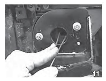
11. Cut the wires flush with the holes so the bumper brackets can be replaced.
