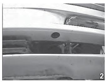
Remove the #12 Torx bolts from below the headlight. Do this on both sides of the vehicle.
