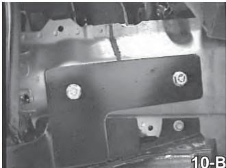
10. Drill the two 3/8" holes for each side of the vehicle using the baseplate as a template. Use the hardware shown in the drawing on page 2 of this document. The wire nut plates are inserted through the front opening of the frame. Tighten according to the chart in the Baseplate General Towing Instructions.
