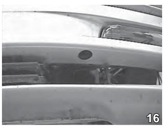
16. The two outside grille pieces need to be removed (snapped into place) to allow the attachment tabs to be used. Keep the pieces for when the cat is not being towed.
