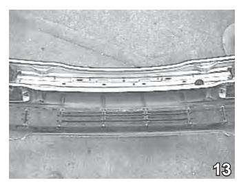
13. Measure the distance between the two holes where the long Torx bolts held the bumper fascia. Set the bumper brackets at the measured distance and hand tighten the bolts.
