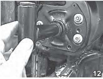
12. Remove the bolts from the front of the baseplate and replace the bumper brackets.
