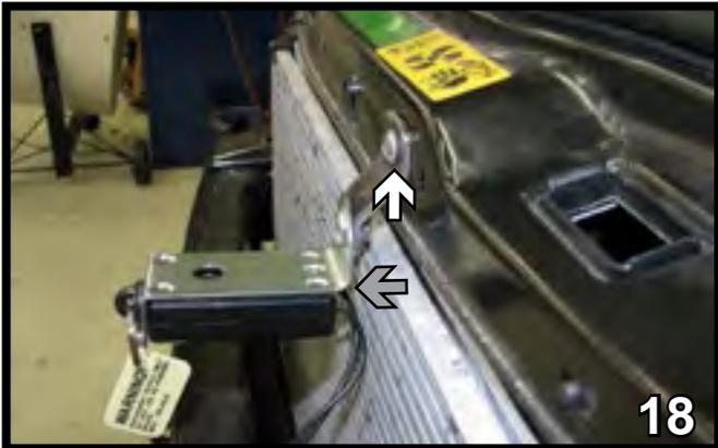
18. Install the breakaway bracket on the front of the frame above the radiator with a 1/4-20 x 3/4" bolt and 1/4-20 nut. Bend the bracket 90° (gray arrow). Attach the breakaway to the bracket using a 1/4-20 x 3/4" bolt and 1/4-20 nut.
