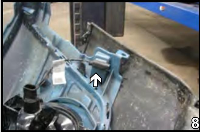
8. Located on both sides behind the grill, there is a temperature sensor that will need to be unplugged.
