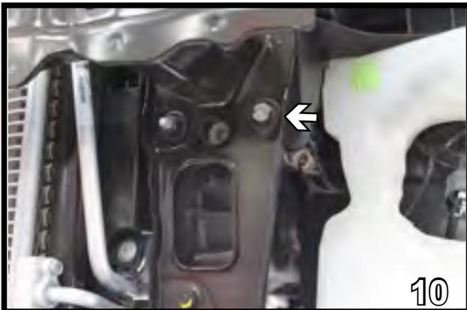
10. Under the reinforcement bumper, use the reciprocating saw to cut the outer bolt off so it is flush with the nut. Do this on both sides.
