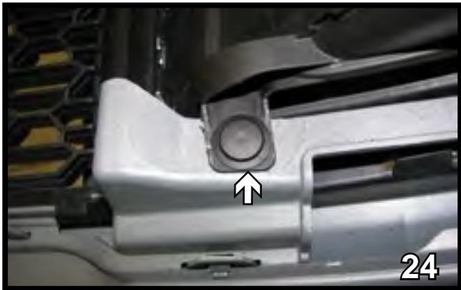
24. **2010 S Convertible:** On the back side of the fascia, the pin had been inserted to come up on this side. Turn it around so that it goes down. Do this to both sides of the vehicle.
