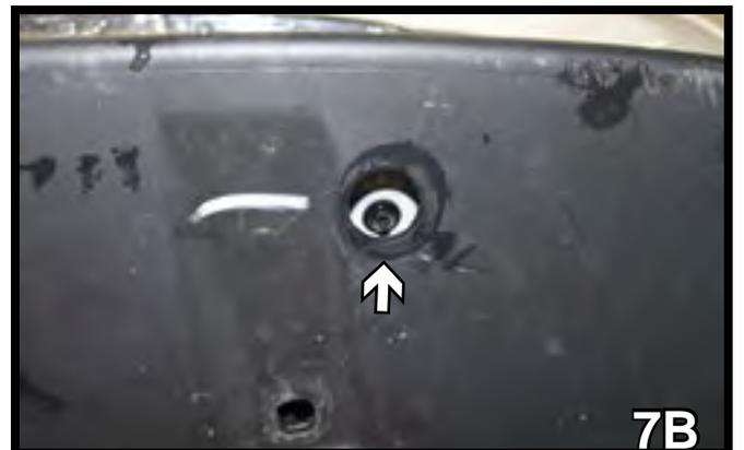
On the 2012 Roadster model there are also three (3) phillips head screws located under cap plugs along the front edge of fascia that need to be removed and set aside.(7B)
