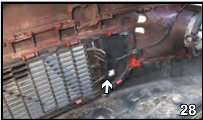
28. **2009 S Convertible:** Make a notch and move the sensor down.
