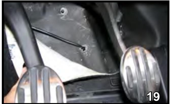
19. Run the brake wire through the floor board under the mat.
