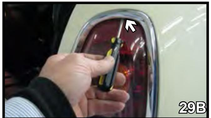
29. Using a flat screw driver, carefully remove the chrome ring around the taillight. Do this on both sides of the vehicle.
