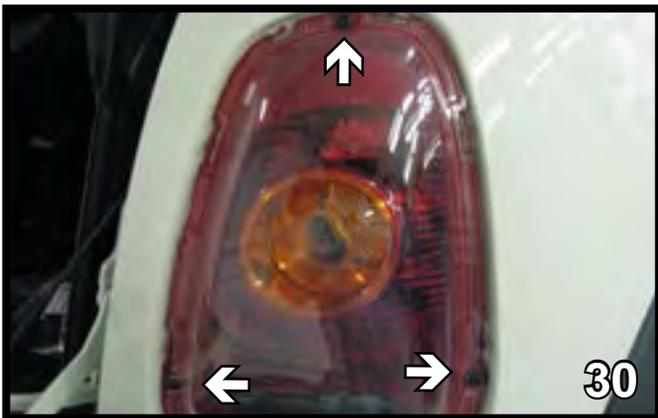
30. Using a phillips screw driver, remove the three screws from the taillight cover. Do this on both sides of the vehicle.
