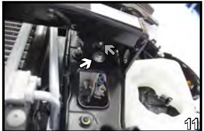
11. Hold the baseplate up in place and start the 8MM-1.25 x 50MM hex bolt (white arrow) with lock and two flat washers into existing hole, make it snug. Using the baseplate as a template, drill the hole above (gray arrow) with a 13/32" drill bit. Do this to both sides.
