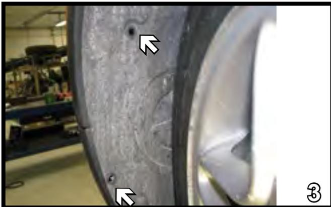
3. Forward of the front tire, use a flat screwdriver to remove two push pins. Do this to both sides. Set push pins aside for later reinstallation.
