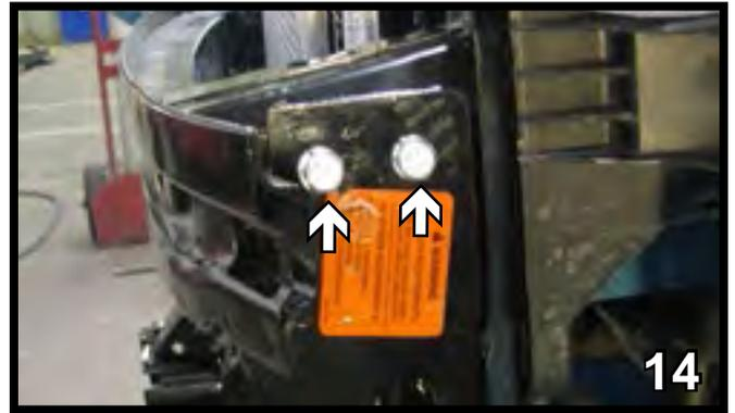
14. Into the holes drilled in the side also insert 3/8"-16 x 1-1/4" bolts with Loctite, 3/8" lock washers and 3/8" nut plates. Do this on both sides.
