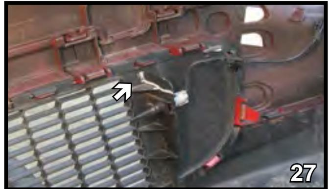
27. **2009 S Convertible:** Continuing on the back side of the fascia, using a utility knife trim down to the gusset and straight out (as shown). Do this on both sides.
