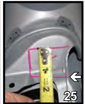
25. **2010 S Convertible:** On the back side of the fascia, using a utility knife trim from the corner down 2" and 1 1/2" wide. Then back up to the point. Do this to both sides of the vehicle. Reinstall the fascia.
