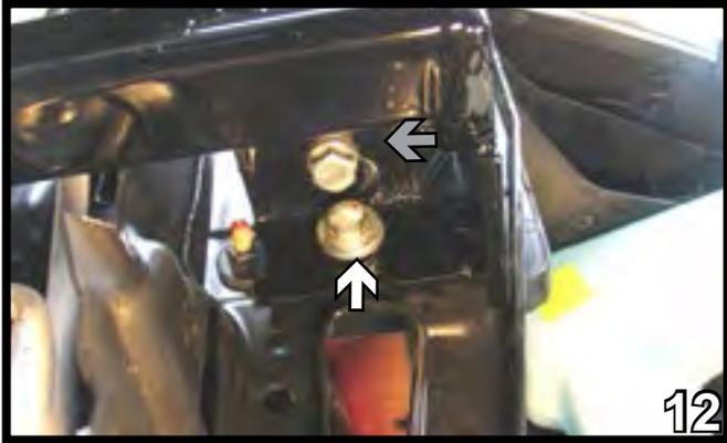
12. Remove the metric bolt (white arrow), replace bolt and washers with Loctite applied. Insert into the top hole (gray arrow) 3/8"-16 x 1-1/4" bolt with Loctite, 3/8" lock washer and tighten to 3/8"-16 nut plate. Then tighten the metric bolt. Do this on both sides.
