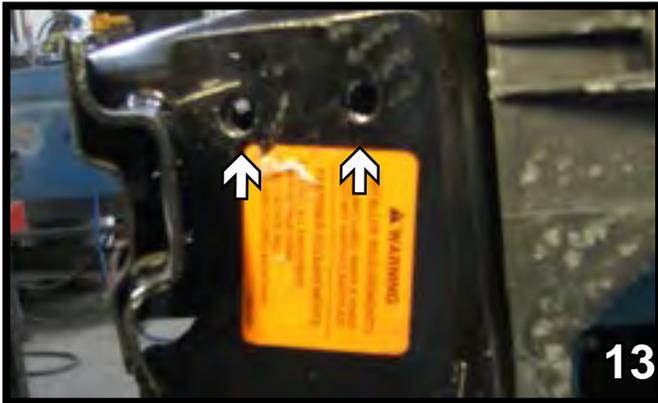
13. Using the baseplate as a template, drill two holes on the side. Do this on both sides using a 13/32" drill bit.
