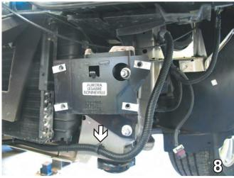
8. Disconnect the cable clamp by pulling it forward through the frame. Move the cable up and out of the way to clear the area for cutting. Do this to both sides of the vehicle.
