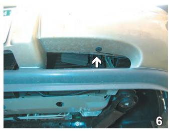
On the lower fascia opening, remove one Christmas tree pushpin. Do this to both sides of the vehicle. Pull fascia forward to remove. Set pushpins and fascia aside to be reinstalled later.
