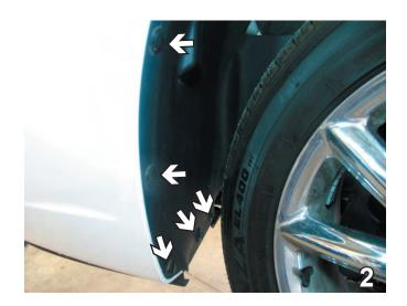
Remove five pushpins just forward of the front tire, on the edge of fascia. Do this to both sides of the vehicle. Set pushpins aside to be reinstalled later.
