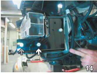
14. Insure crosstube is level. On the lower portion of endplate, forward most hole (see grey arrow), insert 1/2-13 x 1 1/4" bolt and 1/2" lock washer and hand tighten. In the hole next to it (see white arrow), insert 1/2-13 x 1 1/4" bolt, 1/2" lock washer and 1/2-13 hex nut and hand tighten. Do this to both sides of the vehicle.
