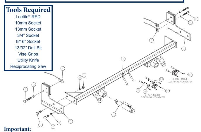
Use only genuine factory replacement parts on your baseplate. Do **NOT** substitute homemade or non-typical parts. If a bolt is lost or in need of replacement, for your safety and the preservation of your baseplate, be sure to use a replacement bolt of the same grade (In most cases it will be Grade 5, please reference the parts list above). Replacement parts may be ordered through your nearest Blue Ox® Dealer or Distributor.
