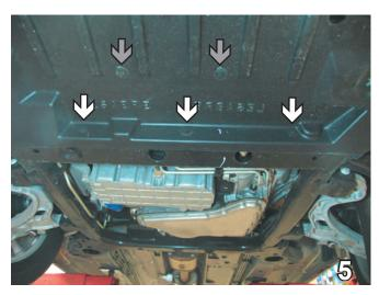
Remove three pushpins near the back of the belly pan (see white arrows). Remove two pushpins near the center of belly pan (see grey arrows). Remove bellypan. Set pushpins and bellypan aside to be reinstalled later.
