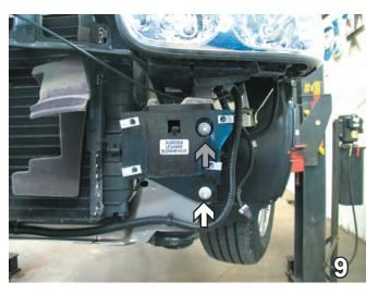
9. Using the 16mm socket, remove the nut from upper section of the bumper bracket (see grey arrow). Pull the nut plate through the side of the bumper bracket and replace nut with the 3/8-16 x 1 hex bolt and 3/8-16 hex flange whiz lock nut. Using the 16mm socket, remove the metric bolt (see white arrow) from the lower section of bumper bracket. It will not be reinstalled. Do this to both sides of the vehicle.
