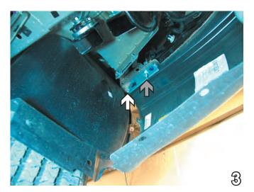
3. Using the 10mm socket, remove one metric bolt (see white arrow) and loosen (do not remove) hex nut (see grey arrow) just forward of the front tire inside the fender well. Do this to both sides of the vehicle. Set bolts aside to be reinstalled later.
