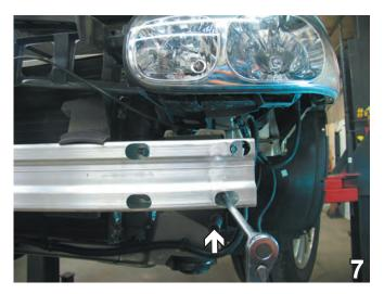
On the metal bumper openings, use the 13mm socket to remove four metric bolts. Do this to both sides of the vehicle. Pull bumper forward to remove. Set bolts and bumper aside to be reinstalled later.
