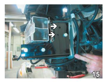
15. On the upper portion of baseplate, use the endplate as a template and drill into the frame using the 13/32" drill bit (see white arrows). Insert 3/8-16 nut plate through frame rail opening and align to drilled holes. Insert 3/8-16 x 1 1/2" bolt and 3/8" lock washer and tighten. Finish tightening all remaining bolts. Trim nut plate wires. Do this to both sides of the vehicle.
