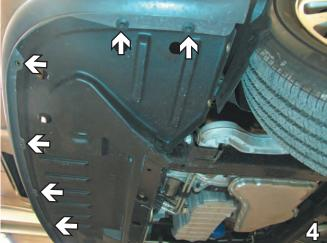
Along the bottom edge of fascia, remove nine pushpins (three on passenger's side not shown). Set pushpins aside to be reinstalled later.
