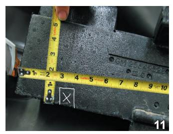
11. With the fascia lying face down and on a soft, flat surface, mark and measure a rectangle on the styrofoam. The rectangle measures 1" x 1". It should be 2 7/8" from the side edge of the styrofoam. Pull the styrofoam from the fascia and lay on a flat surface. Using the utility knife, cut the rectangle 2" deep. Do this to both ends of the styrofoam.
