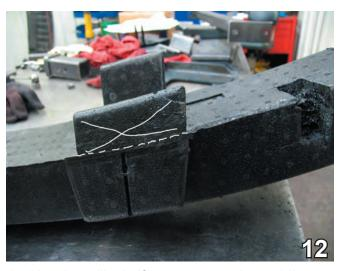
12. Use the utility knife to cut away the molding next to the rectangle just cut so that it is flush with the styrofoam base. Do this to both ends. Place styrofoam back into fascia.
