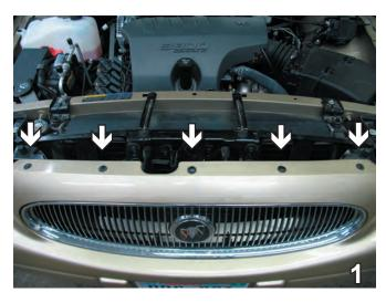
1. On the top of the fascia, above the grille, remove five pushpins. Set pushpins aside to be reinstalled later.
