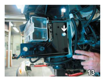
13. Reinstall metal bumper. Align endplate with existing frame rail hole (see white arrow). Endplate should be 1/4" below and parallel to bumper and also parallel with top of frame rail. Insert 1/2-13 nut plate through frame rail opening and align to existing frame rail hole. Insert 1/2-13 x 2 1/2" bolt and 1/2" lock washer and hand tighten to nut plate (don't use Loctite yet). Do this to both sides of the vehicle.
