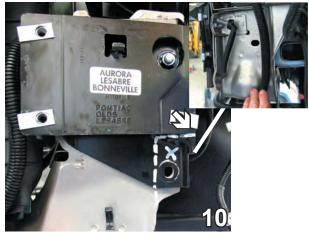
10. Mark a rectangle on the lower portion of bumper bracket. Start horizontally below the upper portion of bumper bracket (see white arrow) and continue just past the lower bolt hole. Then, mark straight down until reaching bottom of frame rail. This vertical marking should be flush with frame rail edge (behind bumper bracket - shown in inset). Using the reciprocating saw, cut marked area through the bumper bracket and frame rail.
