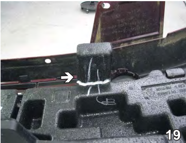
19. On the back side of the fascia, using a utility knife cut off the knobs on the bottom of the styrofoam. Do this on both sides.
