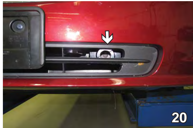
20. Align the fascia to its original position and, using the hack saw blade, trim necessary openings in the grille for the attachment tabs. Do this to both sides of the vehicle.
