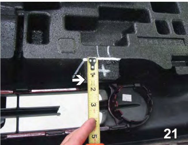
21. On the back side of the fascia in the same area as photo 19, cut the whole lower section off 1 1/2" flush with the bottom of the styrofoam. Do this on both sides.
