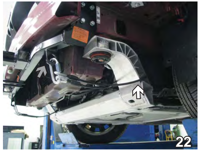
22. Attach the permanent baseplate safety cables to the provided convenience link on the baseplate (see grey arrow). The photo above shows the recommended installation of the permanent baseplate safety cables to frame of the vehicle (see white arrow). Additional options may interfere with suggested mounting, in this case secure the cable to a solid piece of the frame as described in the instructions included with the permanent baseplate safety cables. Be sure the safety cables do not rub against any hoses or moving parts.
