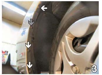
3. Just forward of the front tire, on the edge of the wheel well cover, remove three Christmas tree pushpins, as indicated by the white arrows in the photo above, and one Phillips pushpin, as indicated by the grey arrow in the photo above. Do this to both sides of the vehicle. Set pushpins aside to reinstall later.
