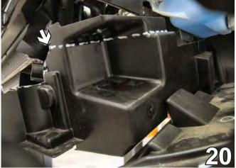
20. On the driver's side, approximately one inch from the top of the air dam, cut horizontally from the front of the air dam to the back.
