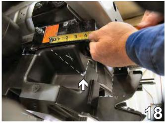
18. On the passenger's side of the air dam, just behind the tab, mark three inches down and two inches horizontally. Then mark upwards, following the contour of the air dam, to the top of the air dam and trim away this area with the utility knife.
