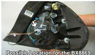
Bulb and Socket Wiring Kit.
