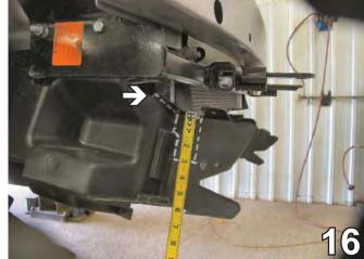
16. Mark the passenger's side of the air dam from the front portion of lip diagonally to the bend and down 3 inches around the contour of the air dam mold. Then mark straight down from the air dam tab three inches and horizontally back to the air dam contour and trim this area wit the utility knife.
