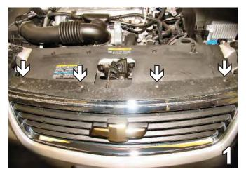
1. Using the Phillips screwdriver, remove four Phillips pushpins from the black plastic cover on the top side of the fascia. Set pushpins and plastic cover aside to reinstall later.
