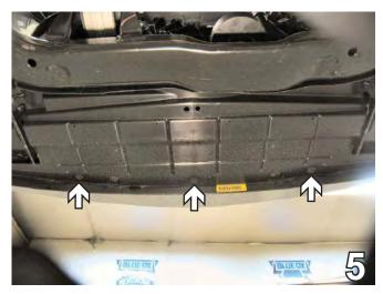
5. Using the 7MM socket, remove three metric bolts underneath the fascia. Set bolts aside to reinstall later.
