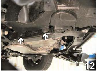
12. Remove two pushpins near the bottom of the wheel well cover on the passenger's side, and one pushpin on the driver's side. Set pushpins aside to reinstall later.
