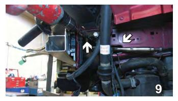
9. Disconnect wiring from area in front of the frame rail. Slide baseplate up so its 1/4" below the top edge of the frame rail and 1/8" away from nut plate built for bumper bracket. Take the vise grips through the hole in the frame and clamp baseplate to frame rail. Then drill all four holes using the baseplate as a template with a 17/32" drill bit. Do this to both sides of the vehicle.
