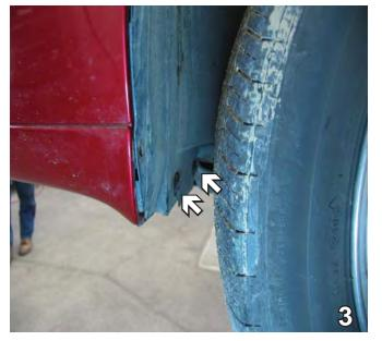
3. Just forward the front tire on the lower edge of the wheel well, remove two pushpins. Do this to both sides of the vehicle. Set pushpins aside to be reinstalled later.
