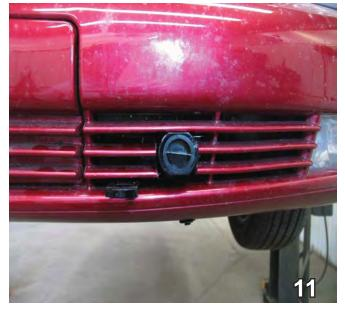
11. Hold the fascia up to its original location. Mark and cut the fascia just on the outside edges of the receiver tube. You should only have to cut the two lower ribs on the fascia. The convenience links should come through the lower opening. Do this to both sides of the vehicle.
