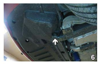
6. Underneath fascia on the back edge of the belly pan, remove one pushpin. Do this to both sides of the vehicle. Set aside to be reinstalled later.
