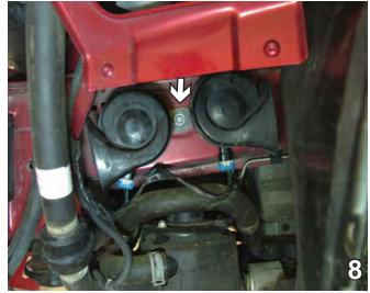
8. Using a 10MM socket, remove the metric bolt on the horn bracket. Set bolt and horn bracket aside to be reinstalled later.
