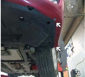
4. Just forward the front tire, on the bottom side of the fascia, remove two pushpins. Do this to both sides of the vehicle. Set pushpins aside to be reinstalled later.
