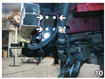
Insert 1/2-13 nut plates through the hole in the frame and align to drilled holes. Insert the 1/2-13x2 1/2" hex bolts and 1/2" lock washers and tighten with 3/4" socket. Trim nut plate wires. Do this to both sides of the vehicle.
