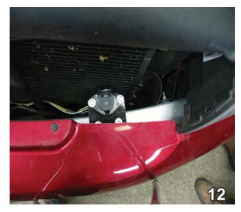
12. Attach electrical bracket to the top of the metal bumper just inside bumper area on the drivers side, using two #10-16x1" self drilling screws and two 1/4" flat washers. Install electrical connector per parts list diagram. 12. Reinstall horn bracket, belly pan, fascia, pushpins and bolts. The baseplate is now installed.
