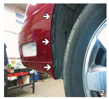
2. Just forward of the front tire, inside the wheel well, remove three pushpins. Do this to both sides of the vehicle. Set pushpins aside to be reinstalled later.
