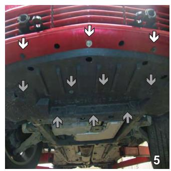
5. Remove three pushpins from the front lower edge of fascia underneath (see white arrows), four pushpins from the center of the belly pan and three christmas trees from the back of the belly pan (see grey arrows). Set pushpins and belly pan aside to be reinstalled later.
