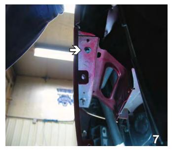
7. Using a 10MM socket, remove one metric bolt from inside the fascia on the corner and loosen (do not remove) two other bolts just forward the first one. Take fascia corner and pull it towards the front of the vehicle, then down and forward again to release it the rest of the way. Disconnect fog and side marker lights. Do this to both sides of the vehicle. Set bolts and fascia aside to be reinstalled later.
