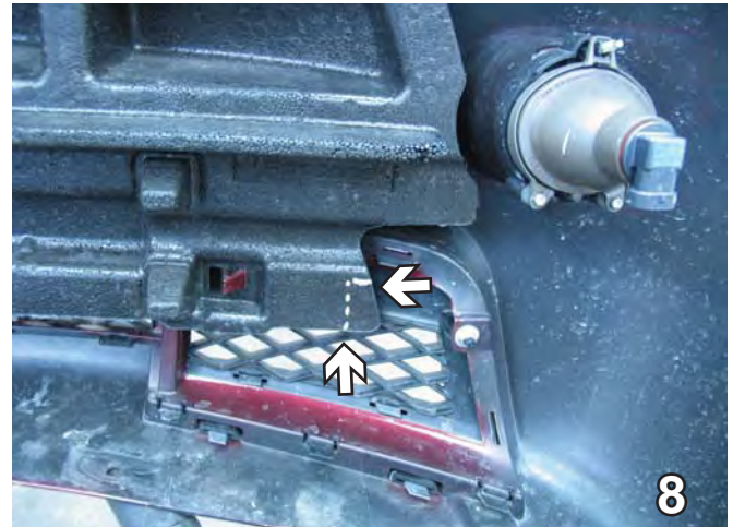
8. Using a reciprocating saw, trim away plastic area, 1" across and up, located on the back side of the fascia.
