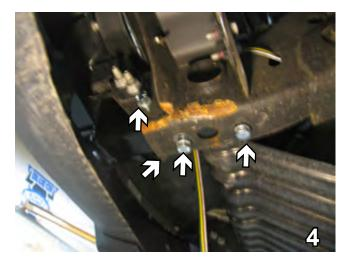
4. Start all four bolts, remount any hole if necessary as every vehicle is different. Insert 1/2 x 1 1/4" hex bolts with 1/2" lock washers. Be sure to use Loctite Red on all bolts. Do this on both sides.
