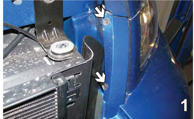
1. Using the 7MM socket remove two 7MM bolts from the front fascia near the headlight housing. This will need to be done to both sides of the vehicle, the driver's side is shown. Set bolts aside to be re-installed later.
