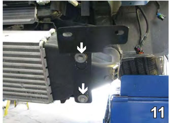
11. With the turbo hanging down, install the new bracket with the existing bolts, starting with the bottom two and tighten. This is done on both sides of the vehicle.
