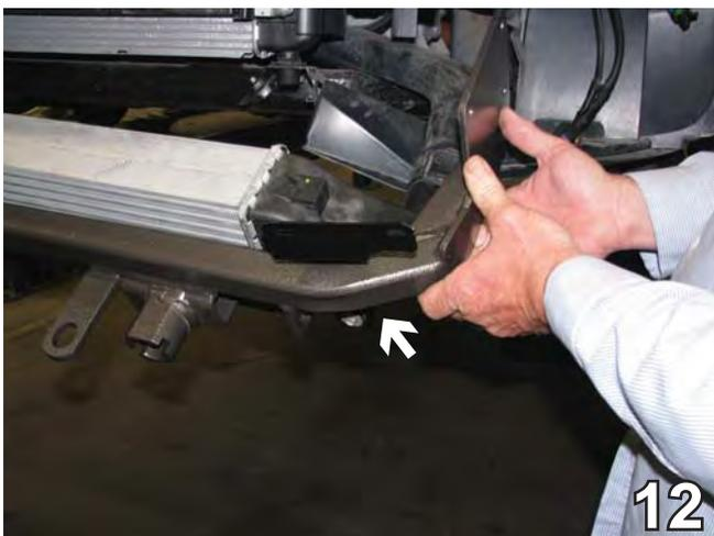
12. Slide the baseplate up underneath the front edge of the turbo. This is done on both sides of the vehicle.
