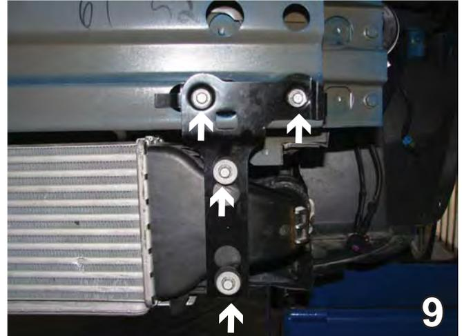
9. This bracket needs to be replaced. Using a 10MM socket, remove the four bolts holding the bracket. This is done on both sides of the vehicle. Set the bolts aside to be used later in reinstalling the new bracket.
