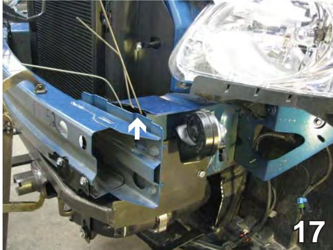
17. Cut the excess wire from the nut plates once they are installed. This is done on both sides of the vehicle.
