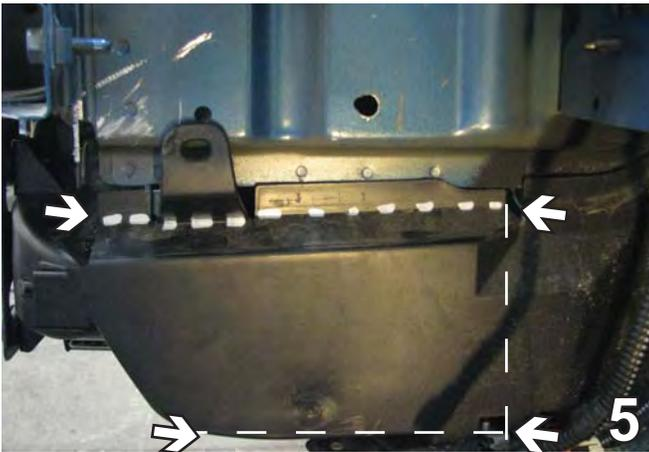
5. Trim the guard horizontally from the edge to the opening on the top and the bottom. Continue trimming connecting the openings vertically. Do this to both sides of the vehicle, the driver's side is shown..
