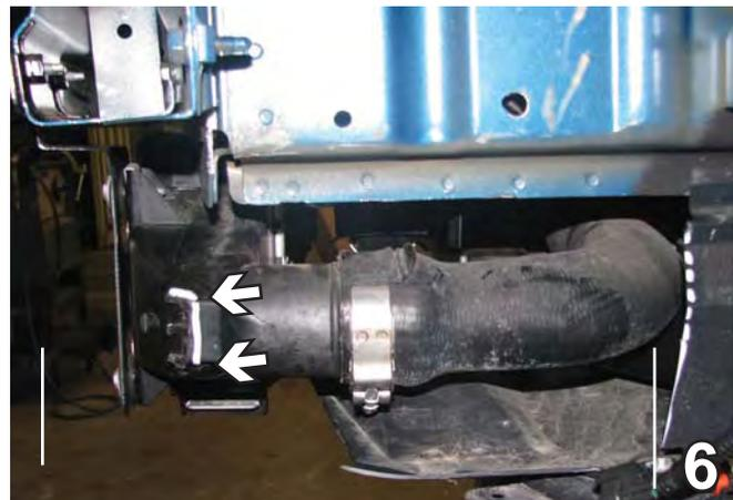
6. Trim the notch off the end of the tube but be careful not to touch anything else. This is done on both sides of the vehicle, the driver's side is shown,
