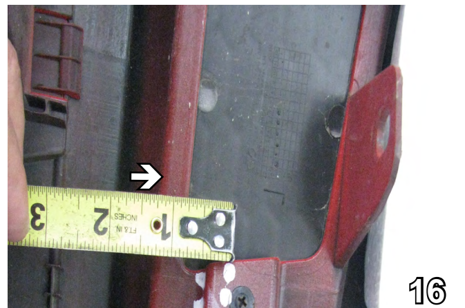
16. On the back side of the fascia, cut 3/8" up from the protruding edge and down to the contour then straight across. Do this on both sides.
