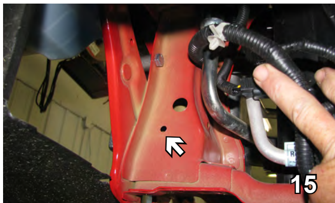
15. On the back of the lower frame extension, undo the hose clip and using the 1 1/4" hole saw drill out the small hole. Do this on both sides.
