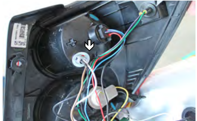
Possible location for the Bulb and Socket Wiring Kit (BX8869).
