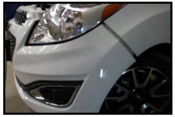
4. Unsnap the fascia at the wheel wells and pull forward to remove fascia from vehicle. Unplug any electrical connections from the fascia and set aside.
