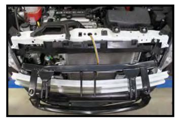
Install the baseplate onto the end plates, using 3/8"-16 hex head bolts and 3/8"-16 nylon lock nuts. Tighten down the baseplate and end plate bolts.
