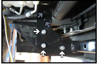
4. Install the side plate on the inside of the frame rail, using 1/2"-13 x 1" bolts, 1/2" lock washers and 1/2" hex nuts (white). Fully tighten the fasteners. Using a 17/32" drill bit, drill the two (2) holes on the inside of the frame (gray). Do this on both sides of the vehicle.
