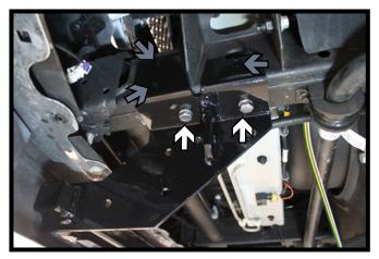
3. Using a 17/32" drill bit, drill the bottom two (2) holes on the frame. Install 1/2"-13 x 1-1/2" bolts with 1/2" lock washers and 1/2"-13 nuts w/wires using the holes in the frame for access (white). Fully tighten the fasteners and remove clamps. Drill the remaining three (3) holes thru the outside of the frame rail (gray). Do this on both sides of the vehicle.
