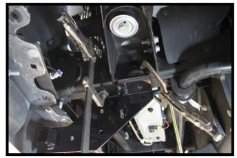
2. From underneath the vehicle, tip the baseplate at a 45 degree angle insert the attachment tabs thru the bumper. Position the baseplate and clamp it to the frame.
