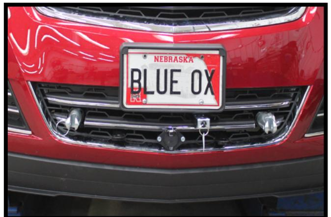
15. Hold the fascia as close to its original position, mark and trim the fascia around the convenience links and attachment tabs. Reinstall the fascia and fascia shroud.
