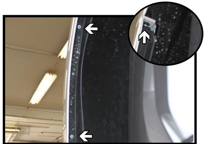
3. **2013 Models:** Using a T20 Torx, remove the three (3) screws from the outer edge of the wheel well. Do this on both sides of the vehicle.
