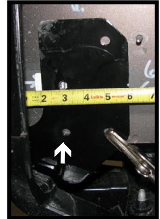
8. Using a reciprocating saw, trim an area on the frame approximately as shown. Cut the bottom flush with the bottom rail (gray) and vertically just inside the rib (approximately 1-5/8") then 2-1/2" back at the top. Do this on both sides of the vehicle.
