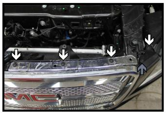
Along the top edge of the fascia, using a T20 Torx, remove the four (4) screws from the driver side (white). Then the three (3) on the passenger side. Using a 7MM socket, remove the screw from the edge on both sides of the vehicle (gray).
