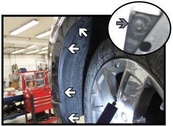
3. Using a T20 Torx, remove the four (4) screws from the outer edge of the wheel well (white). Then behind the wheel well cover, using a 7MM socket, remove the outer screw (gray). Do this on both sides of the vehicle.
