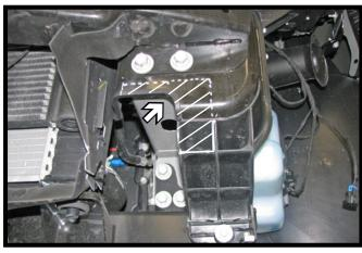
Using a reciprocating saw, notch out the shrouding for baseplate clearance. Do this on both sides of the vehicle.
