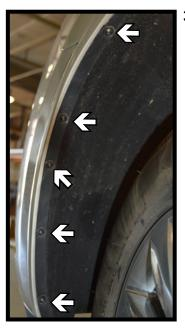
Using a T20 Torx, remove the five (5) screws from the outer edge of the wheel well.
