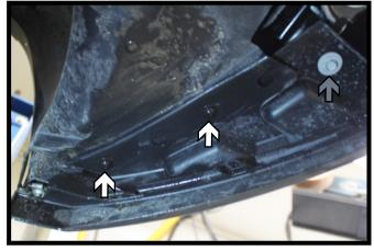
4. On the underside corner of the fascia, using a T20 Torx, remove the two (2) outer screws (white). Then using a 10MM socket, remove the one (1) inner screw (gray). Do this on both sides of the vehicle. Remove the fascia from the vehicle and set aside.
