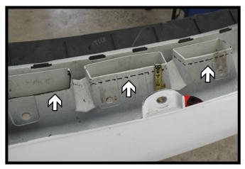
16. Trailblazer Only: On the backside of the fascia, trim the middle three (3) openings approximately as shown for baseplate clearance.
