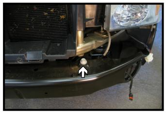
7. Using a 21MM socket, remove the two (2) bolts from the top of the bumper. There is one (1) on each side. Remove the bumper from the vehicle.
