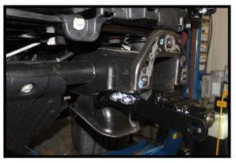
10. Position the appropriate baseplate into the tow hook pocket. Install 1/2"-13 x 5" bolts from the outside of the frame with the convenience link, 1/2" lock washers and lock nuts on the inside of the frame. Tighten down until the frame squeezes against the baseplate. Do this on both sides of the vehicle.
