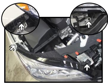
Using a 7MM socket, remove the four (4) screws from headlight. There are two (2) on the top side, one (1) along the side (left inset) and one (1) underneath (right inset). Disconnect the electrical line and set the headlight aside. Do this on both sides of the vehicle.
