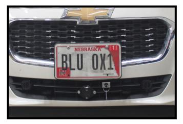
Hold the fascia as close to its original position, mark and trim the fascia around the convenience links and attachment tabs. Reinstall the fascia.
