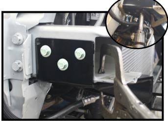
10. Using a 13/32" drill bit, drill the holes in the side plate thru the frame. Install 3/8"-16 x 1-1/4" bolts with 3/8" lock washers into the holes with the side nut plate on the inside of the frame. Do this on both sides of the vehicle. Fully tighten all hardware.
