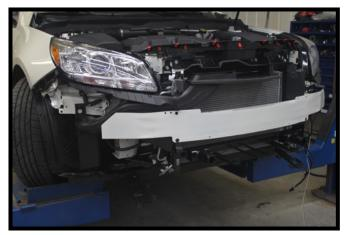
12. Reinstall the bumper, shrouds, baffle, horn assembly and headlights.
