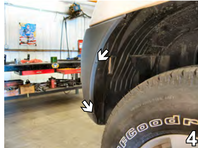
4. Just forward of the front tires on the edge of the front fascia, remove two Phillips screws. Set aside to be reinstalled later. Do this on both sides of the vehicle. The driver's side is shown.
