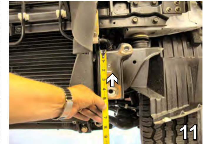
11. Measure down from the top of the frame rail 1 3/4" and center from side to side. Using the 1 1/4" Hole Saw, drill a hole in the frame rail on both sides. The arrow in the picture above illustrates where to drill the hole. Do this on both sides of the vehicle, the driver's side is shown.
