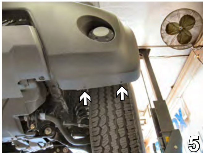
5. Remove two Phillips screws from the bottom edge of the front fascia. Set aside to be re-installed later. Do this on both sides of the vehicle. The driver's side is shown in the picture above.
