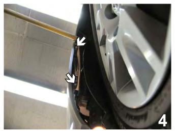
4. Using a 10MM Socket, remove two metric bolts from the inside of the wheel well, just forward of the front tires, and set aside to be re-installed later. This is done on both sides of the vehicle, the driver's side is shown. Pull the front fascia forward and carefully set it aside.
