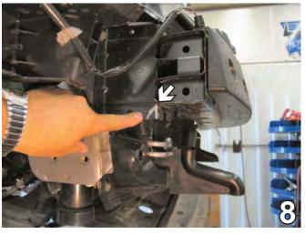
8. On the side of the frame rail extension, behind the bumper, trim a V notch 3/4" back and angled forward to the back side of the front webbing.
