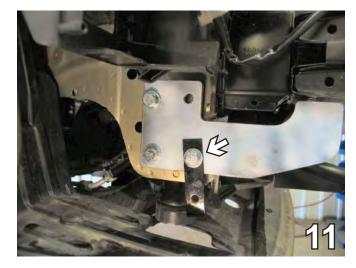
11. On the passenger's side, align the baseplate to the three tie-down bracket holes. Install the two rear 10MM-1.25x35MM Hex Bolts, 10MM Lock Washers and the 3/8 Flat Washers. Insure baseplate attachment tabs are parallel with the ground and the front tie-down bracket hole on the passenger's side is still aligned. Tighten ALL 5 bolts. Be sure that ALL electrical connections are plugged in properly and functioning BEFORE Installing the fascia.
