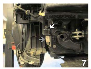
7. Using a reciprocating saw, cut the black plastic under the frame extension bolt horizontally from the outside edge to the frame rail and bend the plastic forward. Finish removing the black plastic by cutting along the bend (white arrow shows trim). The grey arrow shows the webbing which must be bent flush with the frame rail. This is done on both sides of the vehicle, passenger's side is shown.
