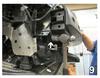
9. Using a hammer, bend the front piece of the frame webbing toward the radiator to relieve the area for baseplate installation.
