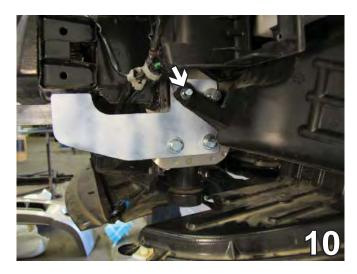
10. On the driver's side, align the baseplate with the tie down bracket holes and fasten it to the frame rail with the 10MM-1.25 x 35MM Hex Bolts, 10MM Lock Washers, and the 3/8 Flat Washers. Do NOT tighten the bolts completely.
