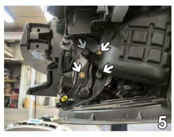
5. Using a 14MM Socket, remove the three metric bolts from the tie-down bracket (see white arrows in photo). This will be done to both sides, the driver's side is shown. On the driver's side remove one bolt from the air baffle using the 10MM Socket (see grey arrow in photo).
