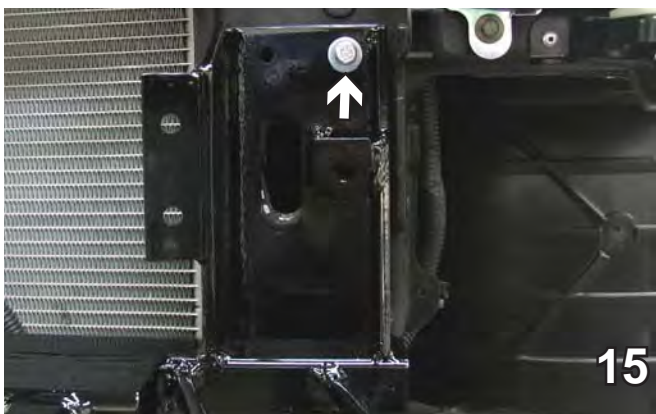
15. To start base plate installation, hold base plate to align with bumper bracket holes, start one bolt on each side. Use 8MM hex bolts and 5/16" flat and lock washers.
