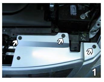
Remove three push pins from the top of the front fascia and set aside to be re-installed later. This is done on both sides, the driver's side is shown.
