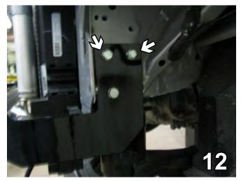
12. Insert 1 1/2" hex bolt and 3/8" lock washer into the top two holes and fasten to a 1" nut plate inserted through the opening on frame end. Use Loctite Red and torque to specifications. Do this on both sides.
