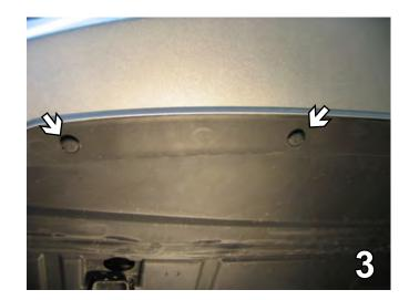
3. On the underside of the front fascia there are five push pins that need to be removed as indicated by the arrows in the picture. Set these aside as they will be re-installed later.
