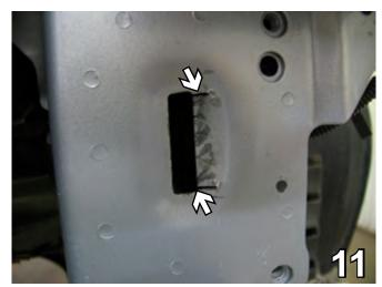
11. Using a reciprocating saw make a cut at the edge of the opening, bend the metal cut in. Do this on both sides.
