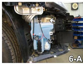
6. On the passenger side, remove the three metric bolts from the windshield washer reservoir with a 10MM Socket. Release the two wire clips from the electrical wires, then disconnect and plug the hose. Set all aside to be reinstalled later.
