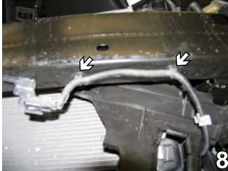
3. Unplug the sensor by pulling the tabs out of the lower bumper.
