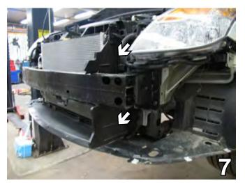
7. Remove the black plastic from above and below the frame extension by pulling it out. This is done on both sides of the vehicle.
