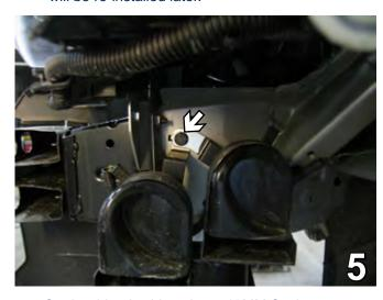
5. On the driver's side using a 13MM Socket, remove the metric bolt from the horn. Unplug and set aside to be reinstalled later.
